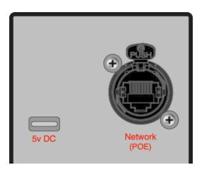
Power & Network - OSCA can be powered by POE IEEE 802.3 or 5v DC via the USB C port
